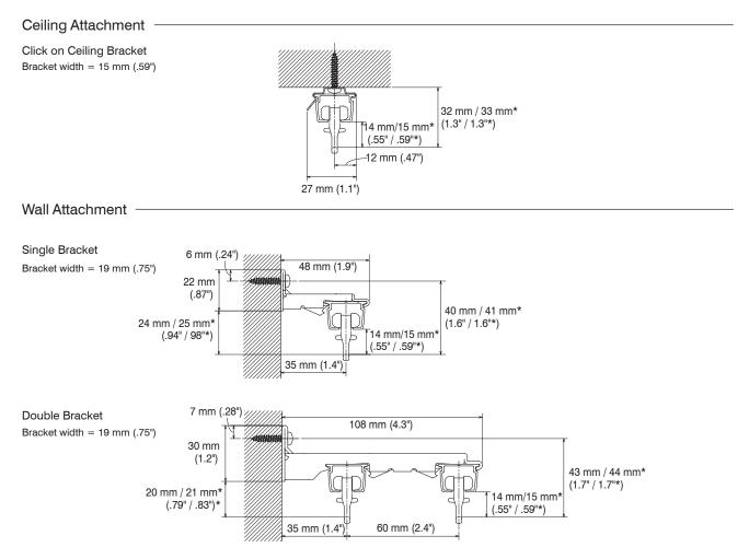
\*Measurements apply to use of New Delac Rollers or Nexty Rollers.
